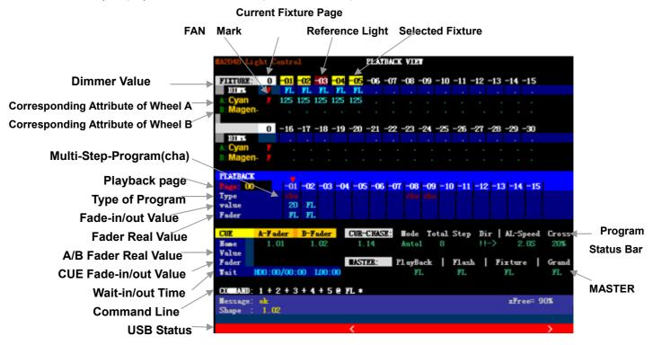
MA3000 Intelligent Fixture Controller is displayed on VGA1 monitor and also on VGA2 monitor, through which, output value of channels of DMX singal from controller can be displayed. (Shown as graph)
