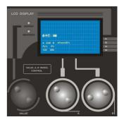
2) A Wheel/B Wheel is primarily used to set various attribute values of fixture.
