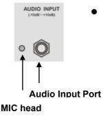
Audio signal can be taken from mixer controller, line level output of other audio equipments, or MIC input. Controller automatically extracts low-frequency component from music as music trigger synchronous signal for Multi-Step-Program program.
