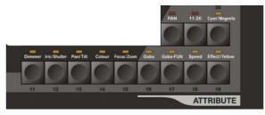
10 attribute keys correspond to the attribute labeled above respectively. Pressing "11-20" Attribute Switch key (indicator light is on) means switched to 10-20 attribute key. One attribute key includes two attributes, which means a total of 40 attributes of intelligent fixture can be controlled through Attribute Switch key.
